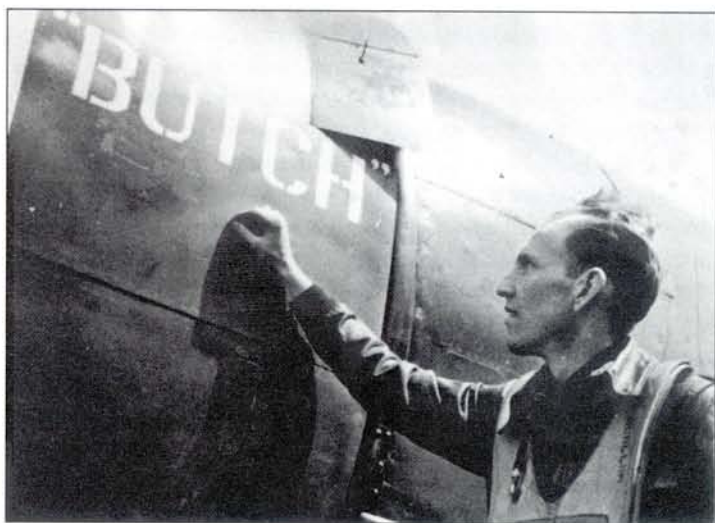
The early ‘short’ cowling flaps that identified the widely used P-47C are shown above ‘Mac’ McCollom’s personal aircraft in the 4th FG (via M Bowman)
