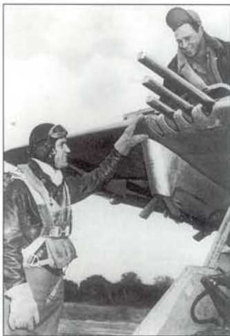
With the panels removed, the right hand Browning machine guns on Johnson's P-47 are given a routine check by Sgt Penfold
