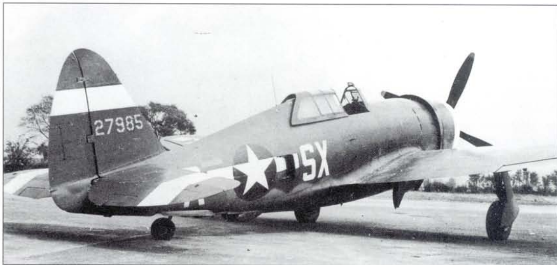
This P-47D-2 was assigned to the 352nd FS/353rd FG. Photographically the 'poor relation' of VIII Fighter Command, the 353rd nevertheless produced five full P-47 aces. Note the whip, rather than mast, aerial fitted to this particular batch of Thunderbolts
